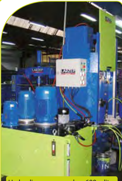
Hydraulic powerpack, 600 litre capacity with 3 different pumps to work at different pressures and flows.
