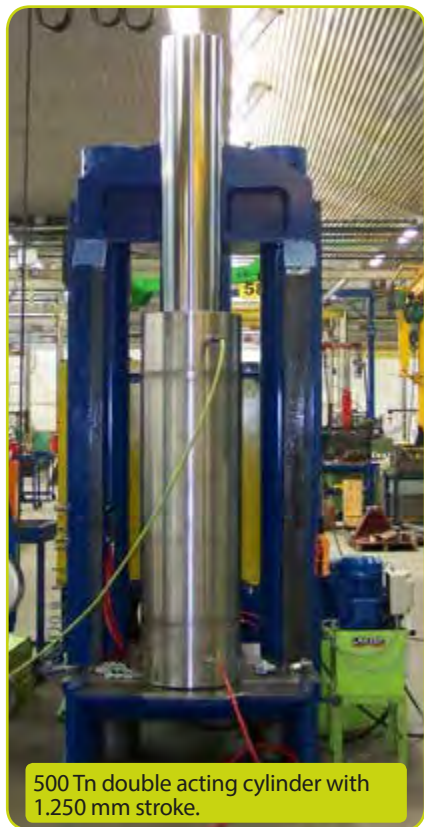
Double acting cylinder with motorized lock nut and gear wheel.
